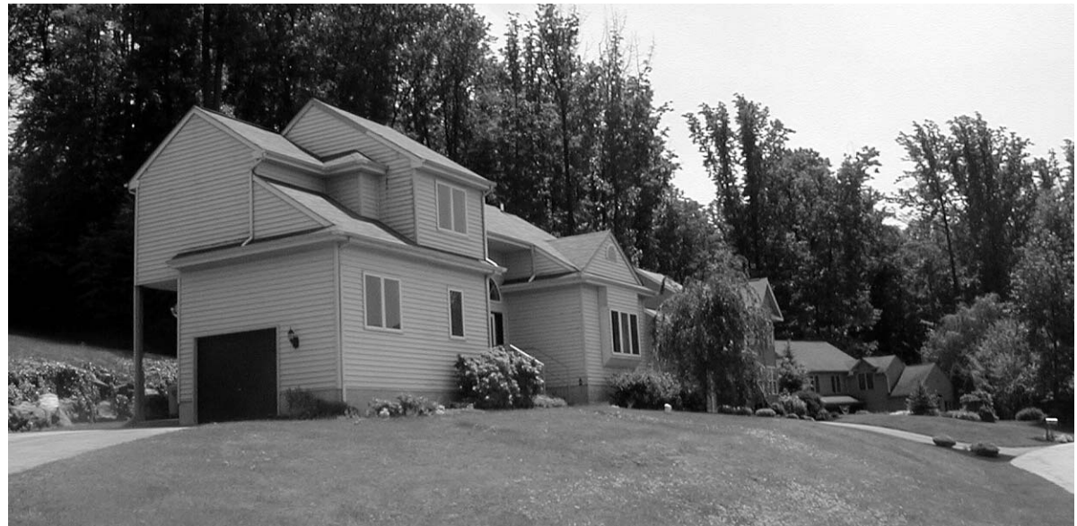
Side-load garages reduce the visual impact of garage doors on the house facades.
