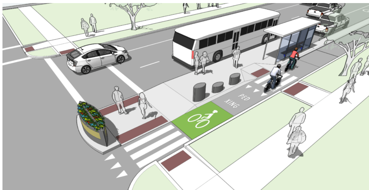
Conceptual rendering showing the incorporation of a bus stop into a protected bike facility.
