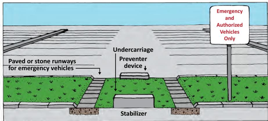
An efficient system that prevents misuse is the use of grass paver which provides a stabilized surface. This allows for grass to grow in the crevices and over the pavers so that they cannot be seen. In most cases they do not require a chain.
