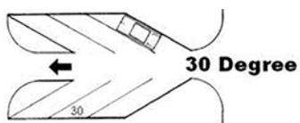
**Angled—30 Degree** – Similar to 45 degree configurations, this configuration progressively increases the amount of pavement required per space while narrowing the double bay cross section. Standard dimensions for this configuration are 9 foot wide by 16.5 foot deep spaces with a 12 foot wide (one-directional) driveway aisle for a total 45 foot wide cross section.
