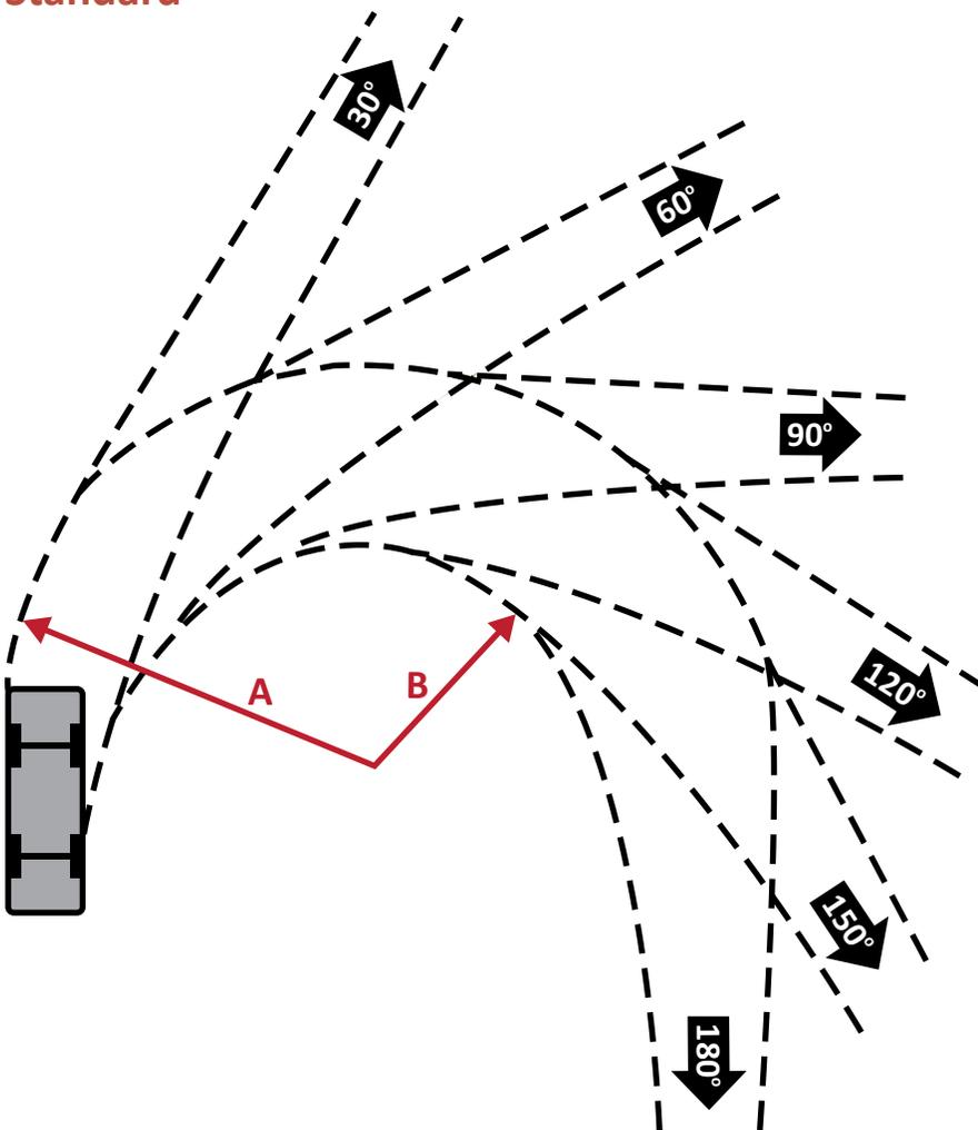
Please refer to the chart on the following page for the Minimum Design Turning Radius (A) and Minimum Inside Turning Radius (B) values.
