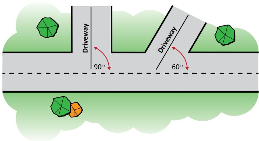
*The angle of a driveway is measured from the centerline of the roadway to the centerline of the driveway.*
