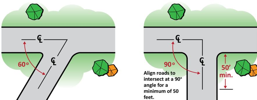
Align roads to intersect at a 90 degree angle for a minimum of 50 feet.
