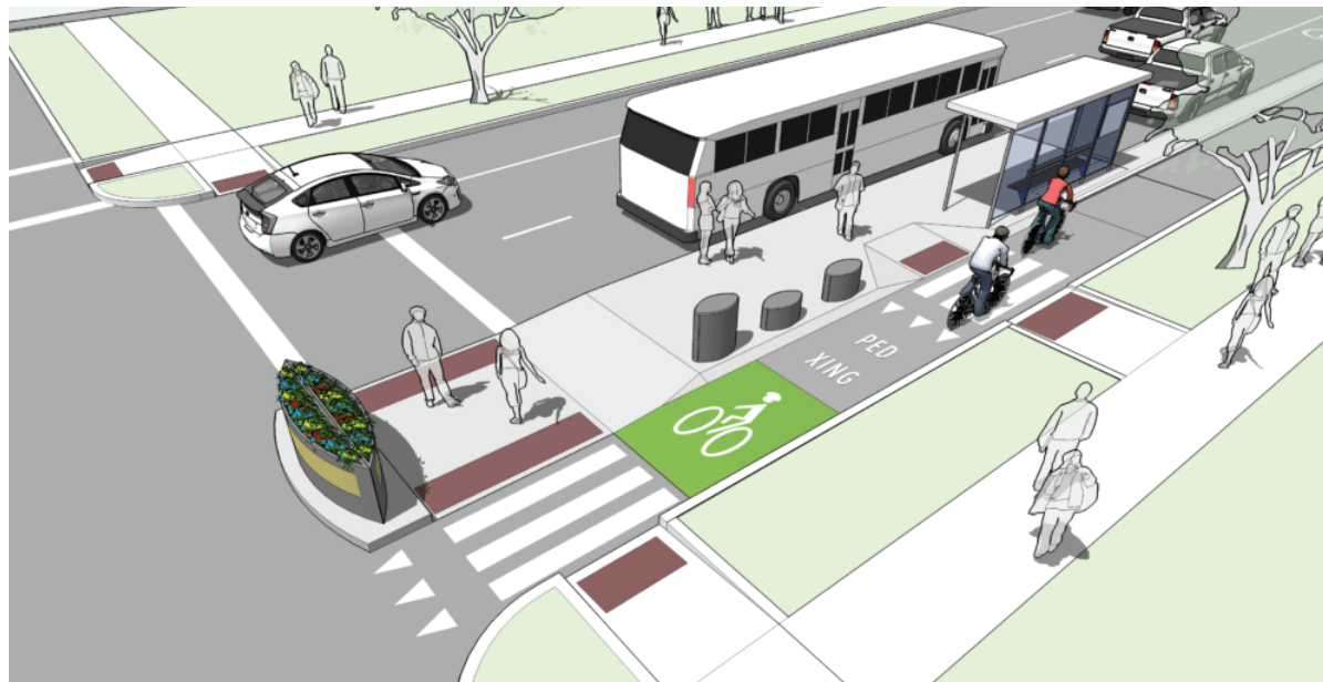
Conceptual rendering showing the incorporation of a bus stop into a protected bike facility. Source: Alta Planning + Design.
