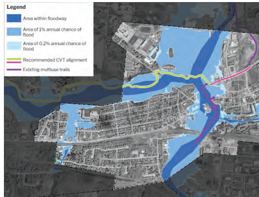
The recommended alignment passes through floodways and flood plains in Downingtown Borough and may require special design treatments and permitting.
